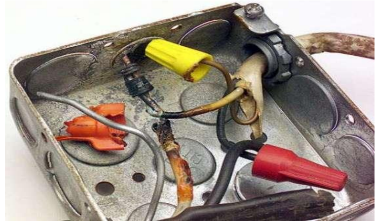
BURNT CABLES IN A JUNCTION BOX
